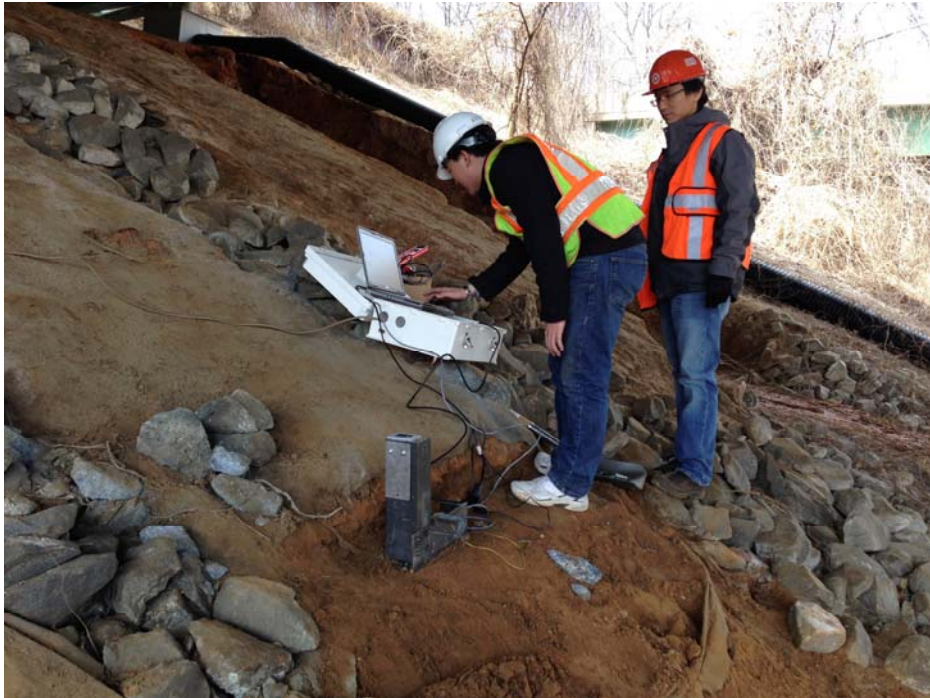
Figure 6 - Laser distance sensor to measure deflection of Girder #2 of I-95 Bridge
