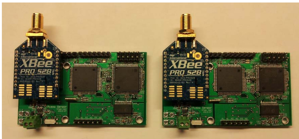
Figure 7 - Soldered Wireless Piezoelectric Sensor PCB
