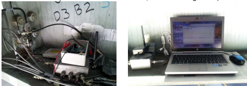
Figure 19 Test Platform (Left: Wireless Piezo Sensor, Right: Base Station and Laptop)
