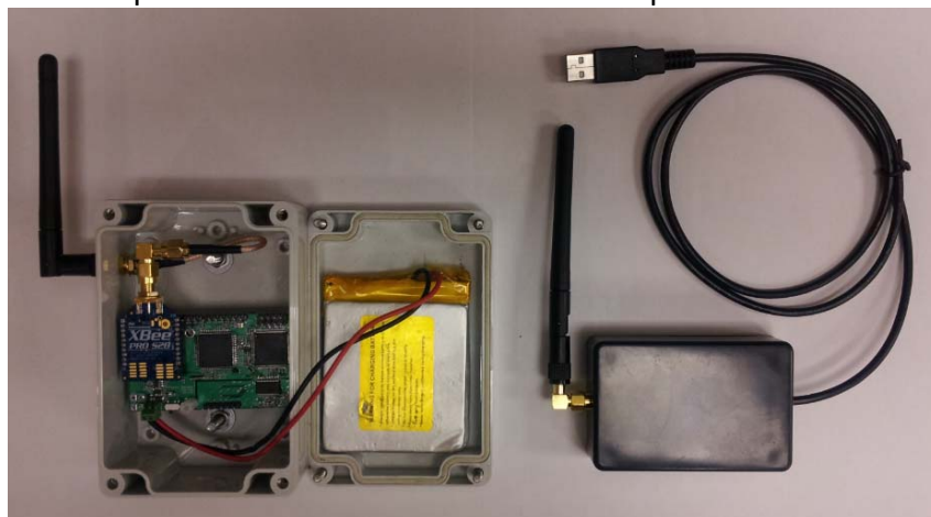
Figure 1 Redesigned Wireless Piezoelectric Sensor (Left) and Base Station (Right)
