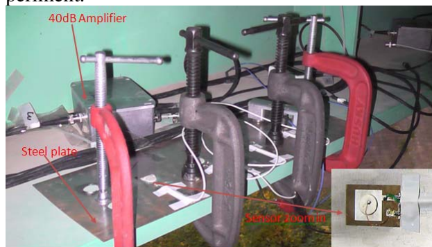
Figure 4. Steel plate with four sensors mounted on the lower flange of the I-girder bridge
