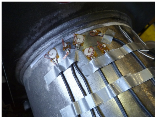
Figure 5. Piezo film AE sensor array (left) and Relation between cumulative AE signal counts (hits) and loading cycles of the fatigue test
