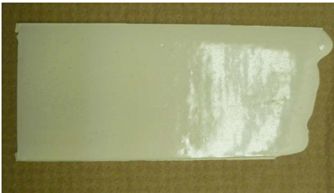
Figure 6. Picture of a large piezo paint patch (size about 2 x 5 inches) made in our lab for sensor fabrication
