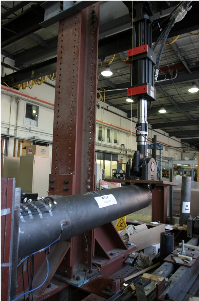
Figure 3 - test setup for fatigue testing of full-scale steel tube from traffic signal post
